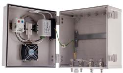
The AccelTex Solutions Heated & Cooled PoE enclosure allows an access point to be installed in an outdoor or other temperature-limiting environment. The heater, fan and AP are all powered by a single PoE cable run from the network switch. The enclosure ships ready for an AP and external antenna installation.
